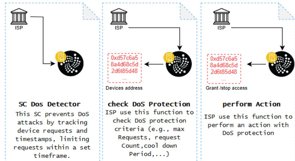
**Figure 8.** The workflow of the DoS Detector SC along with the actors involved in IOTA.
