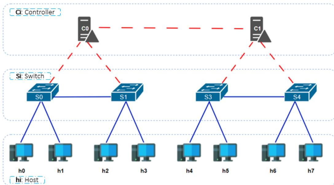
**Figure 10.** Topology of our system for securing SDN based on IOTA 2.0.
