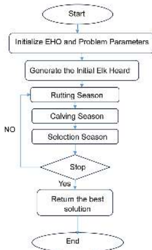
Fig.1. Flow chart for EHO algorithm.
