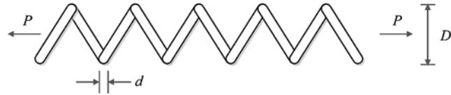
**Figure 17:** Schematic of the tension/compression spring design
