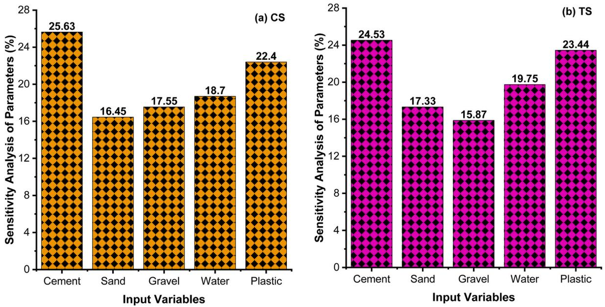
Fig. 17. Outcomes of sensitivity analysis (a) CS and (b) TS models.
