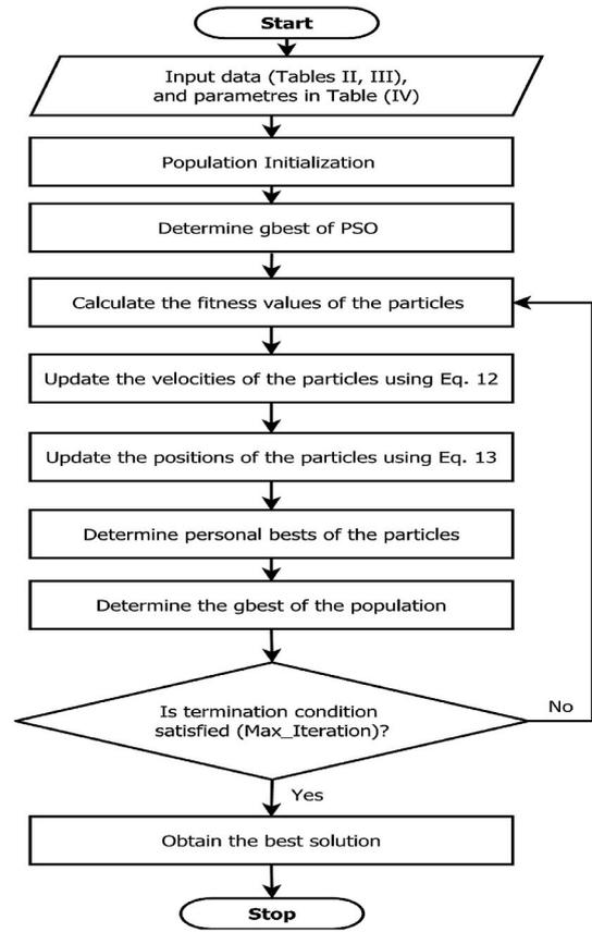
Fig. 7. Flowchart of proposed approach using PSO.
