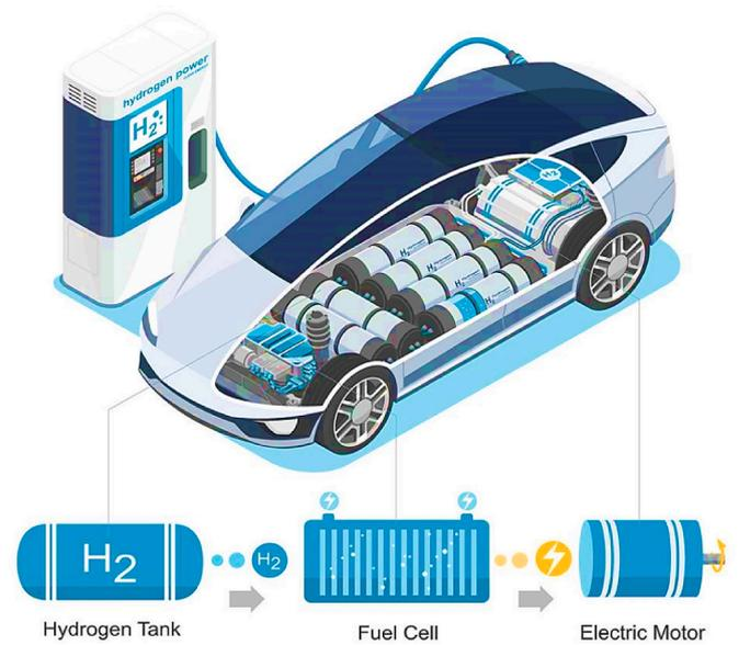
Fig. 2. Fuel cell of Hydrogen vehicle with Station Ecology.
