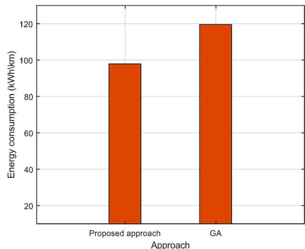
**Fig. 13.** Comparison between the proposed approach and GA due to energy consumption.
