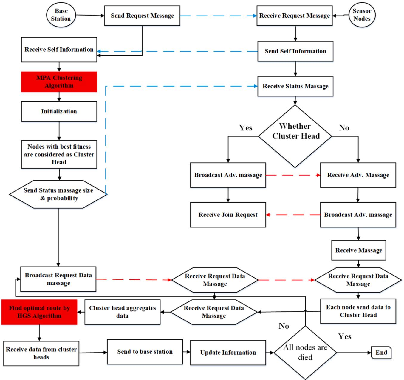
Fig. 3. The HGS-MPA Block diagram.
