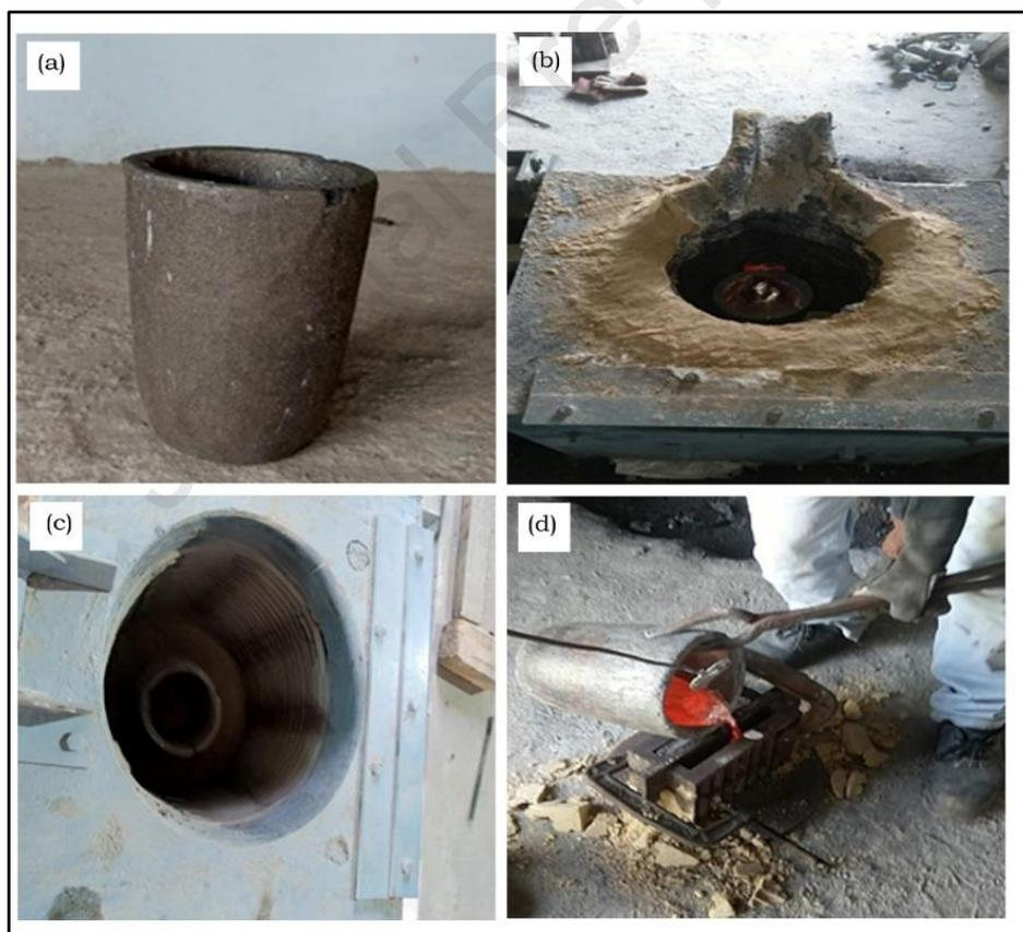
Fig. 2. Stir casting of AA2014, AA6061 with 5%WC and 5%Al<sub>2</sub>O<sub>3</sub>
