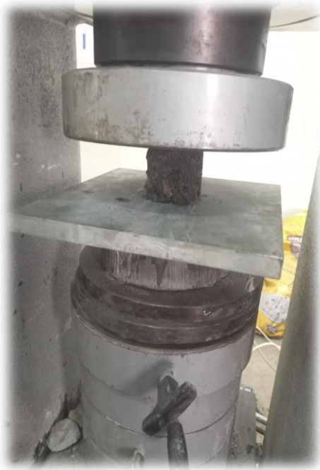
Fig. 3: Compressive strength testing
