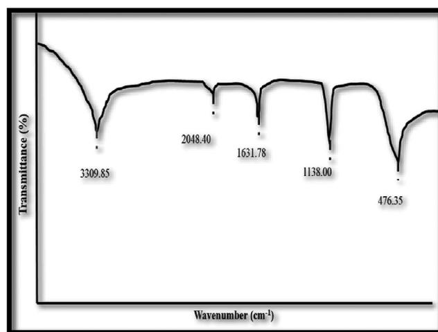
FIGURE 2 | FT-IR nanoparticles of silver spectra.
