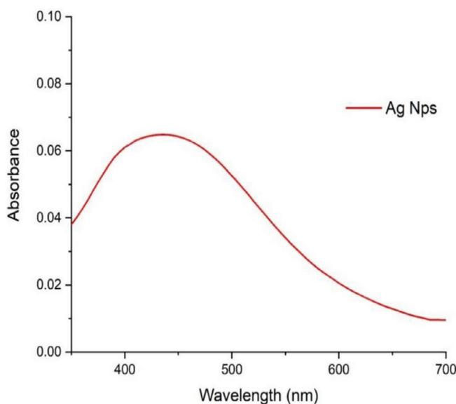
FIGURE 3 | UV-vis spectrum of green synthesized silver nanoparticles.
