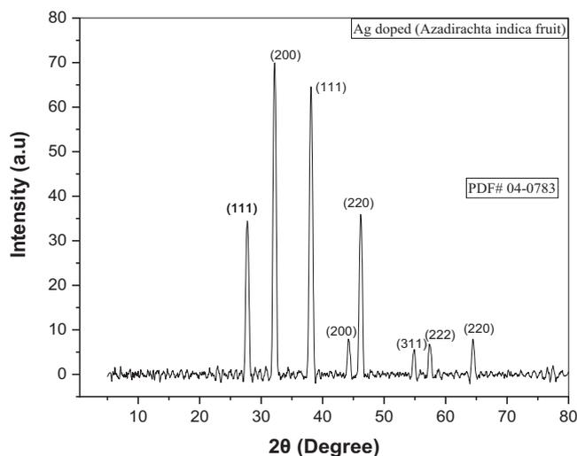
FIGURE 1 | X-ray diffraction (XRD) analysis of green silver nanoparticles.
