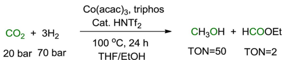
Fig. 5 Cobalt-catalyzed hydrogenation of \text{CO}_2 to methanol (Kar et al. 2018a). Copyright 2017, Elsevier B.V. (License number: 5886450667058)
